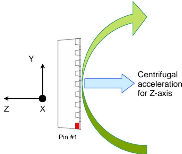
Figure 22. Centrifugal acceleration applied for SCA3000 Z-axis.
