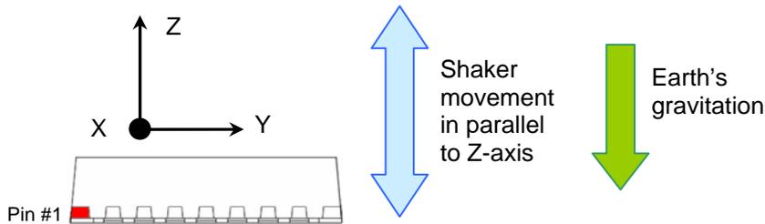
Figure 24. SCA3000 movement in Z-axis bandwidth measurement.
