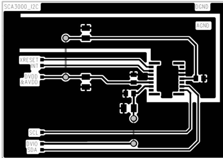
Figure 19. Recommended PWB layout for SCA3000 with I<sup>2</sup>C interface (not actual size, for reference only).
