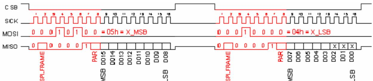
Figure 7. An example of SPI read communication.
