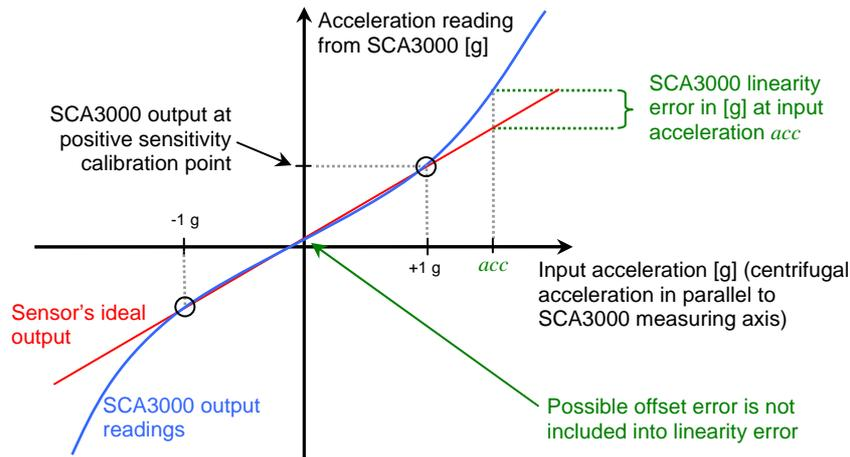
Figure 23. SCA3000's linearity error at input acceleration  $acc$ .
