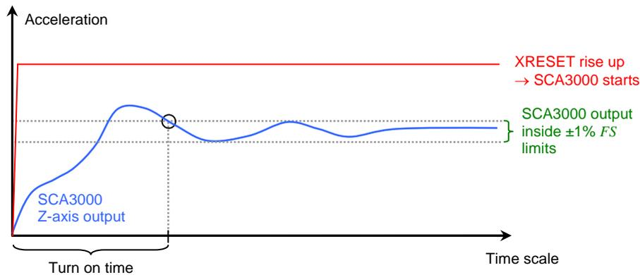
Figure 25. Turn-on time definition for one axis.
