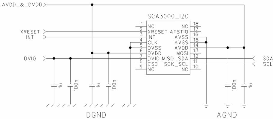
Figure 16. Recommended circuit diagram for the SCA3000 with I<sup>2</sup>C interface.
