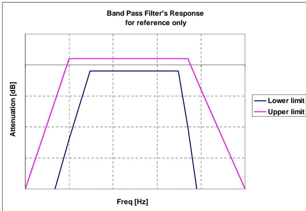
Figure 2. The MD band-pass filter's frequency response.
