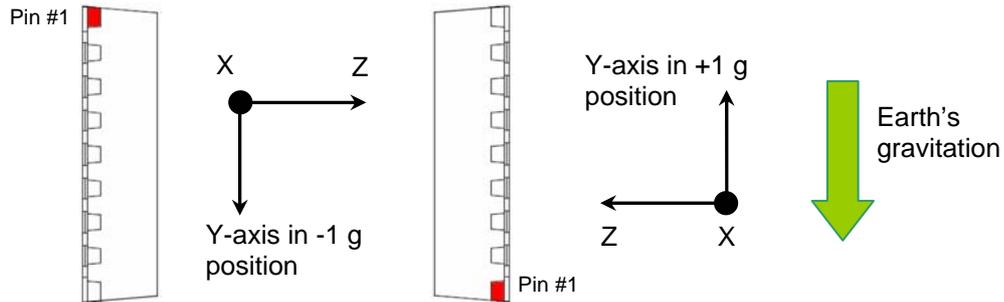
Figure 21. SCA3000 positions for Y-axis sensitivity measurement.
