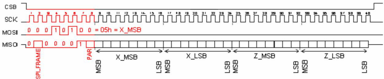
Figure 8. An example of decremented read operation.
