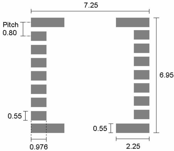
Figure 17. Recommended PWB pad layout for SCA3000.
