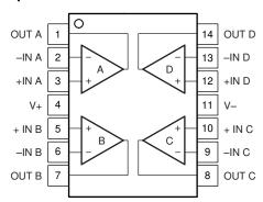
Figure 5-5. OPA4140: D (14-Pin SOIC) and PW (14-Pin TSSOP) Packages, Top View
