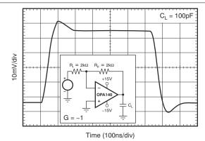
Figure 6-27. Small-Signal Step Response (100 mV)
