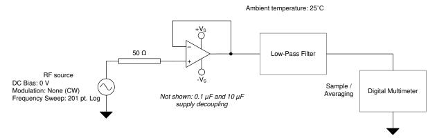
Figure 7-7. EMIRR +IN Test Configuration
