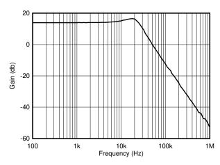
Figure 8-2. OPAx140 Second-Order, 25-kHz, Chebyshev, Low-Pass Filter
