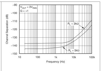
Figure 6-32. Channel Separation vs Frequency
