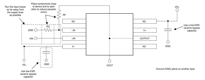
Figure 10-1. Operational Amplifier Board Layout for Noninverting Configuration
