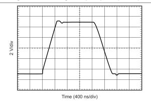
Figure 6-29. Large-Signal Step Response
