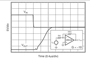
Figure 6-23. Positive Overload Recovery
