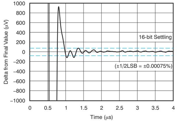
**Figure 6-26. Large-Signal Negative Settling Time (10-V Step)**
