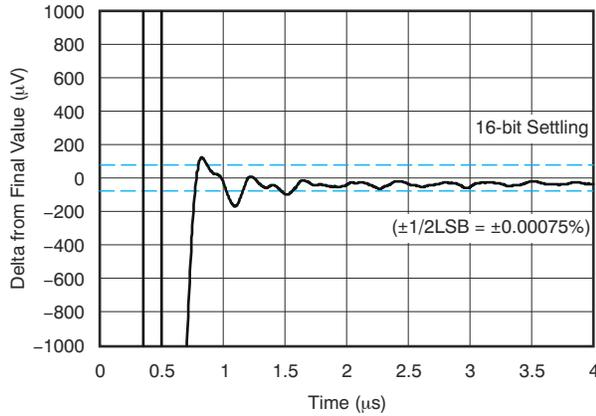
**Figure 6-25. Large-Signal Positive Settling Time (10-V Step)**
