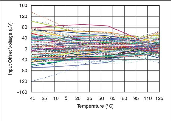
**Figure 6-4. Input Offset Voltage vs Temperature (144 Amplifiers)**
