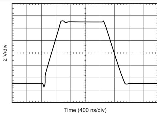
**Figure 6-29. Large-Signal Step Response**
