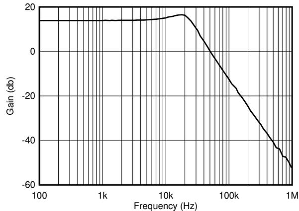
Figure 8-2. OPAx140 Second-Order, 25-kHz, Chebyshev, Low-Pass Filter
