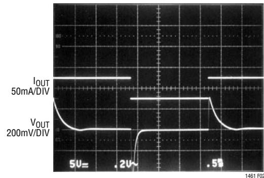
Figure 2. 50mA Load Step with  $C_L = 2\mu\text{F}$
