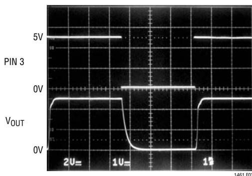
Figure 3. Shutdown While Delivering 25mA,  $R_L = 100\Omega$
