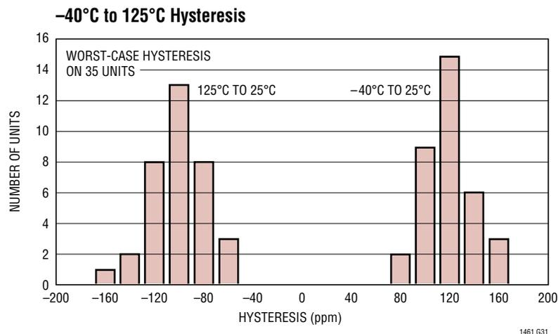
**TYPICAL PERFORMANCE CHARACTERISTICS** Characteristic curves are similar for most LT1461s. Curves from the LT1461-2.5 and the LT1461-5 represent the extremes of the voltage options. Characteristic curves for other output voltages fall between these curves and can be estimated based on their output.
