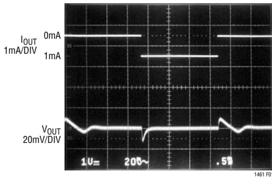
Figure 1. 1mA Load Step with  $C_L = 1\mu\text{F}$
