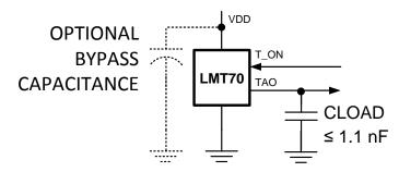
Figure 24. LMT70 No Isolation Resistor Required
