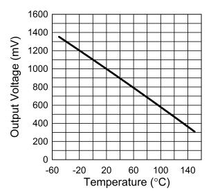
Figure 23. LMT70 Output Transfer Function
