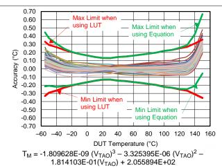
Figure 30. Using Third Order Transfer Function Best Fit -10°C to +110°C
