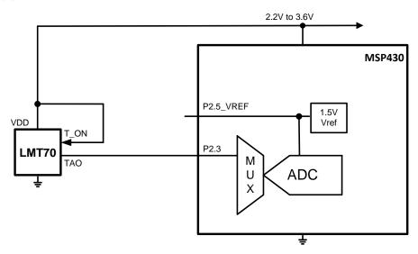
Figure 26. Typical Application Schematic
