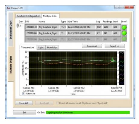
Disable autoscale to zoom in on a desired region. The mouse wheel does not work to zoom, instead, highlight the time and type in a new value, then click with the mouse somewhere on screen to accept the new value.
