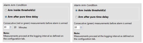
**Alarm Arming Delay:** Within threshold = How many in-bounds readings required to arm the alarm. Pure time delay = The number of log intervals to wait before arming the alarm.
