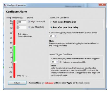
**Note:** System-level warnings and failures take precedence over user-defined threshold alarms, so if any LEDs are blinking on USB connect, it's a good idea to open software and see what happened.
