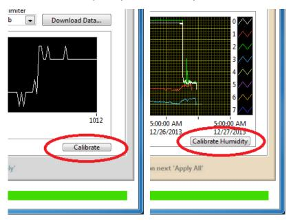
This is the calibration section of Otero. There are no parameters to calibrate Temperature or Light, so the calibration option will only appear if one or more Digit-TLH are connected to the computer.
