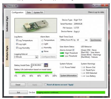
**Log Interval:** The rate at which data is collected. If the environment is changing rapidly, you may choose to take a reading every 10 seconds. Or, if the environment is more stable, a log interval of 10 minutes may be all that is necessary to capture a good data set. Requires Apply.
