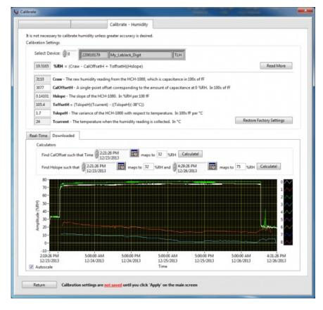
The raw humidity value (Craw) is a measure of capacitance in hundreds of fempto Farads. To convert humidity from fempto Farads into a %RH, use the following equation.
