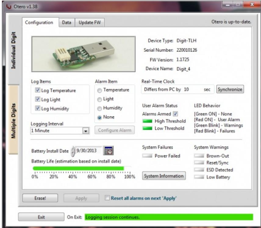
**Log Interval:** The rate at which data is collected. If the environment is changing rapidly, you may choose to take a reading every 10 seconds. Or, if the environment is more stable, a log interval of 10 minutes may be all that is necessary to capture a good data set. Requires Apply.
